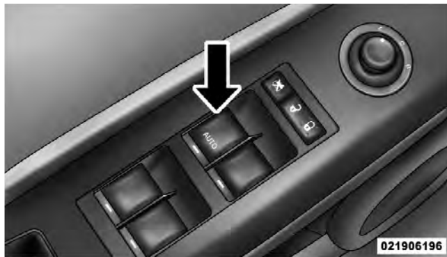
Power Window Switch Location
